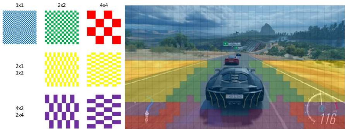
Figure 32. Turing VRS Supported Shading Rates and Example Application to a Game Frame
